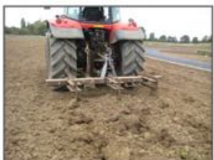
Plate 2: Tractor drawn subsoiler
