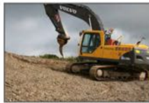
Plate 3: 360 with Single Rigid Tine Attachment
